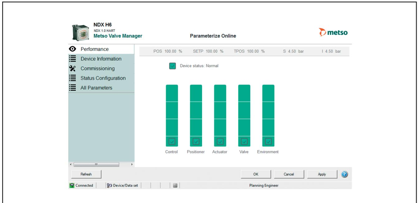
Fig. 2. The Performance View of the Metso Valve Manager graphically displays indexes of the valve, actuator and positioner, as well as indexes of control performance and the application environment. Report will show explanations of the status of each component and guidelines for recommended actions.
