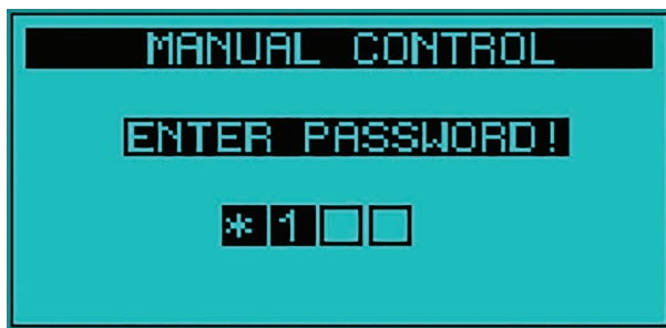
Figure 29: Manual control password entrance screen
