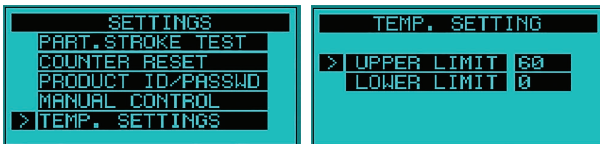
Figure 31: Temperature limit setting tab
