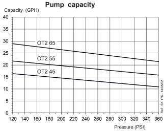
Viscosity = 5 cSt - Rated speed = 3450 rpm
